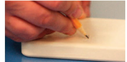
The pencil test is a simple field test to identify the durability of the powder coated finish. By writing on the surface with a pencil and wiping it off, it is easy to compare hardness, cure, and resiliency of the finish.
