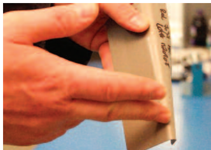
The Mandrel Bend uses a uniform bend on a metal part to test the flexibility of the finish. Powder formulations can be modified to adjust for flexibility or hardness needs.
